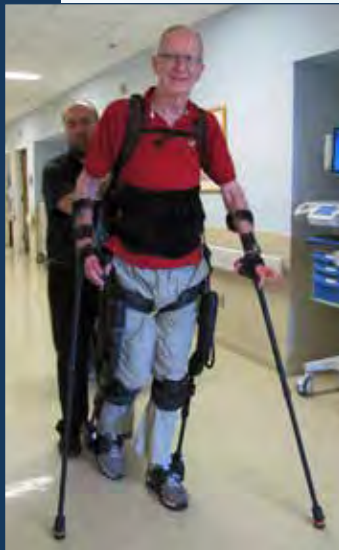
U.S. Marine Corps Veteran William Lehman walks in the Ekso exoskeletal-assisted walking device under the supervision of study staff.
