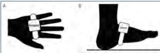
Experimental setup. (A) Participants wore inertial sensors on the dorsum of the hand, wrapped around the 2nd to 5th metacarpal bones. (B) Foot sensors were placed on the dorsum of the foot.
